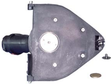
Abb. 29 Knife head without circular knife
