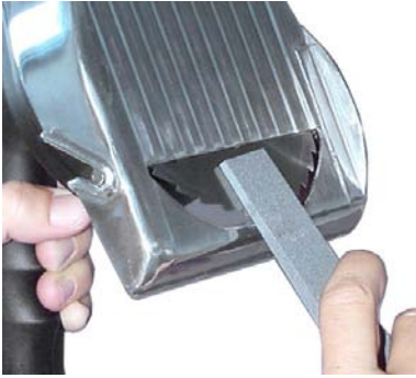
Abb. 49 Deburring the circular knife
