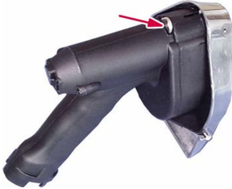
Abb. 15 Knurled screw for setting the cutting depth
