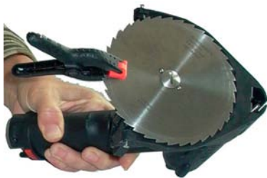
Abb. 28 Circular knife fixed with gripping device
